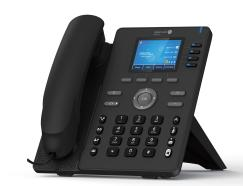
The H6 DeskPhone can fit up to 4 lines of text, and support up to 1000 contacts and call logs. The phone also comes with a multi-angle adjustable stand designed to meet user needs across various scenarios.
